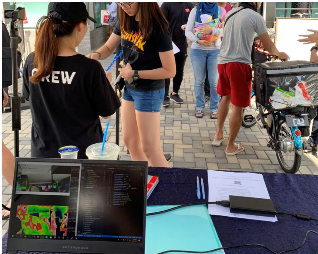
Figure 22: SPOTON can take the temperatures of groups of up to 10 people in real time
